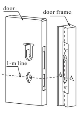
Remarks: 1. Position and size of the holes must be confirmed before cutting.
