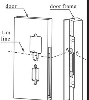
Remarks: 1. Position and size of the holes must be confirmed before cutting. 2. If there is shock absorption bar on door frame, its thickness should be excluded from door thickness.
