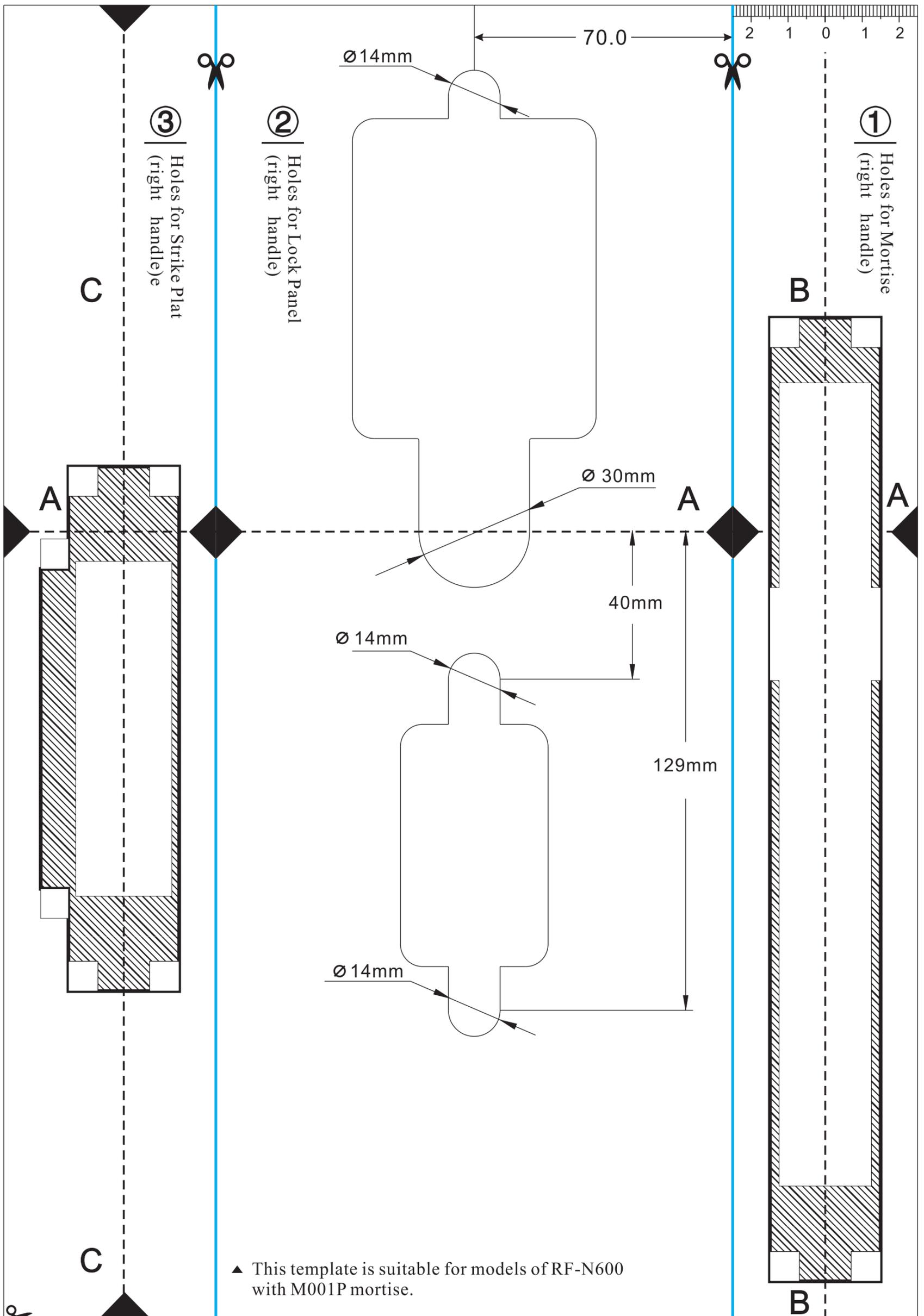
▲ This template is suitable for models of RF-N600 with M001P mortise.
