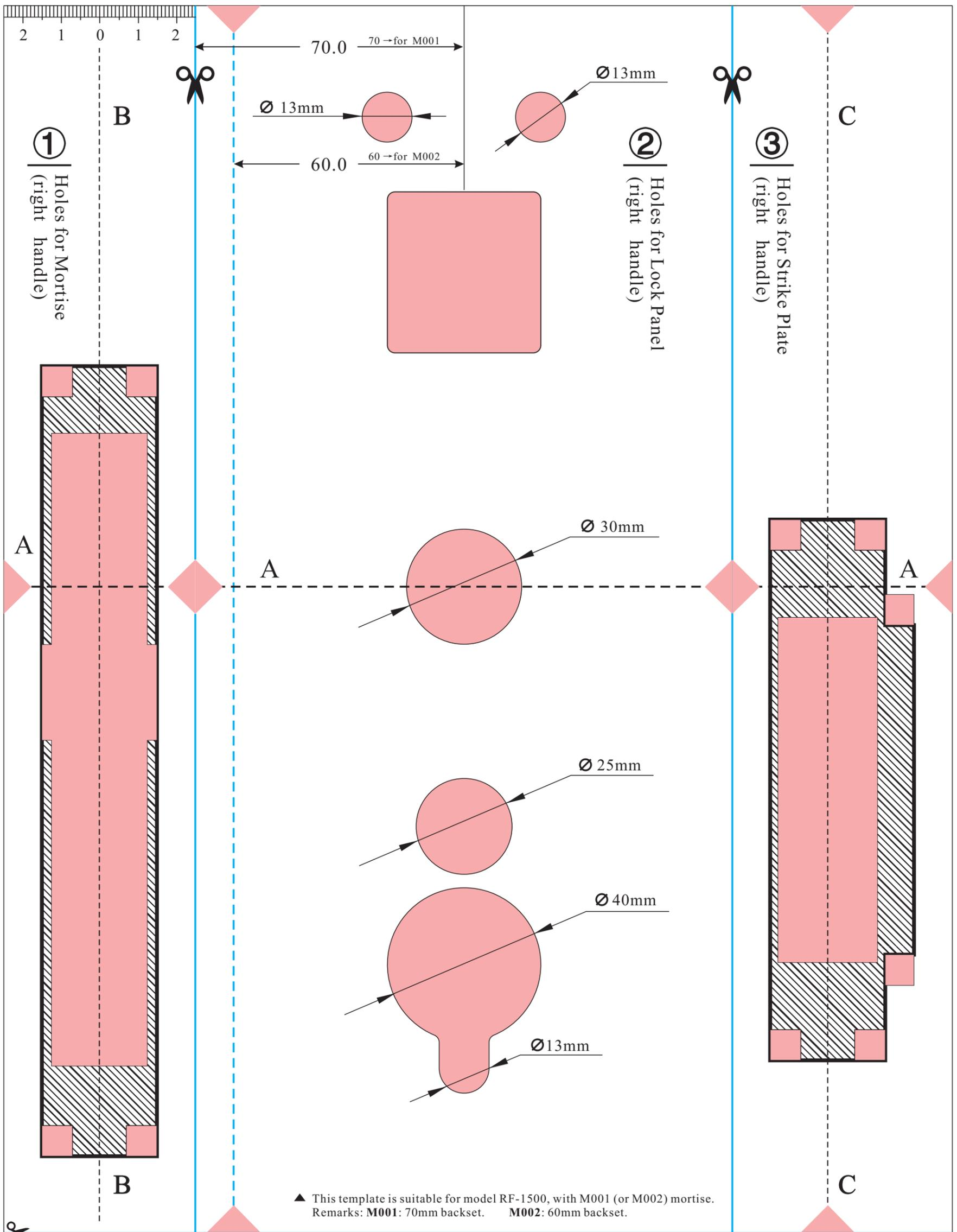
▲ This template is suitable for model RF-1500, with M001 (or M002) mortise.
