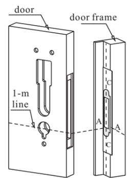
Remarks: 1. Position and size of the holes must be confirmed before cutting. 2. If there is shock absorption bar on door frame, its thickness should be excluded from door thickness.
